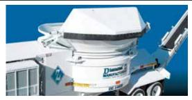
Allows safe operation of a Diamond Z tub grinder in an environment where horizontal and other designs are not permitted. With its combination of deflector shield and containment shield, the Diamond Z Containment System controls up to 99.9% of all ejected material/thrown debris. A standard feature in all Diamond Z tub grinders.
